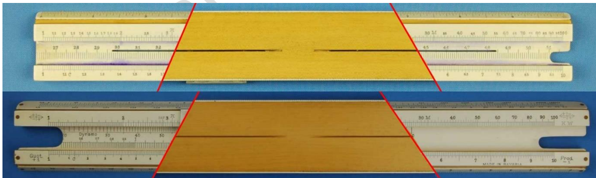
Figure 13: Stock slits; front/back \ front of typical non-electro model with wood and celluloid cut through (top), and electro model 368 with only the wood cut (bottom).
