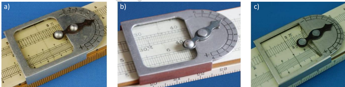
Figure 10: Digit-registering cursor rivets; a) two domed, b) one domed and one flat, c) two flat.
